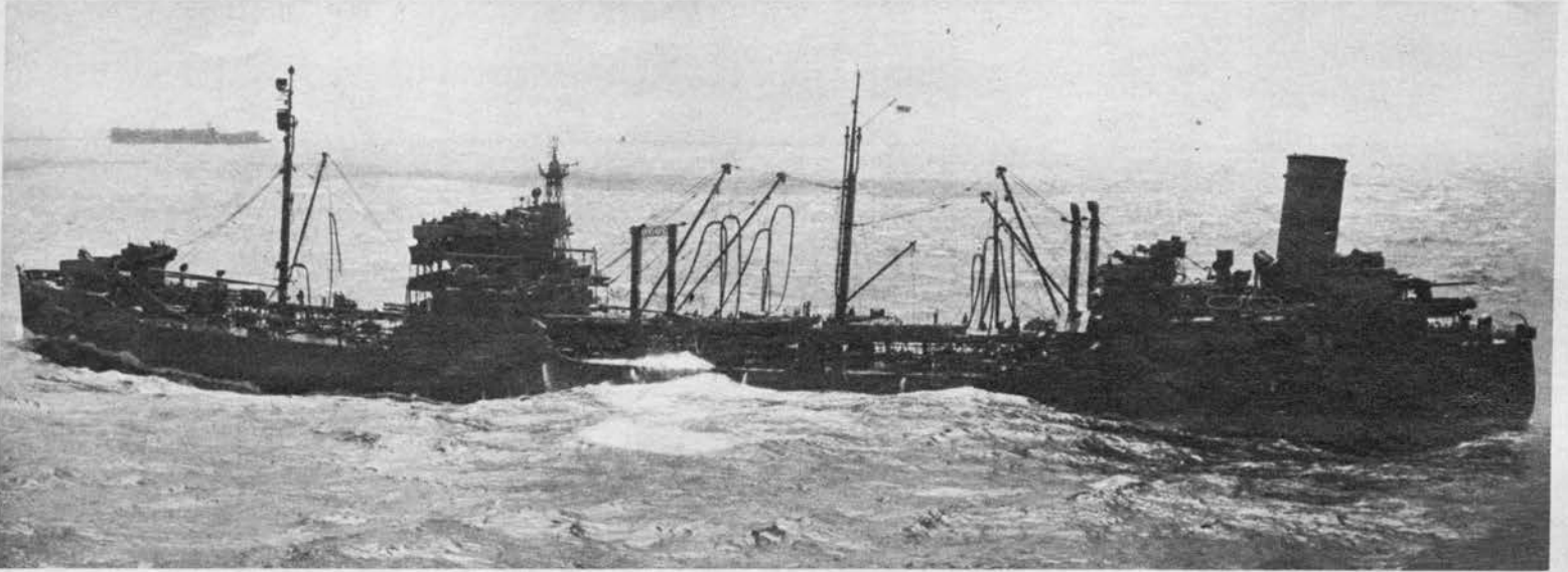
Fleet oiler of USMC T-2 design is hauling in her pumping hose after refueling a cruiser. Observe how waves break over her weatherdeck as she rides low. Fast, long-range T-2 tankers are designed to follow the
